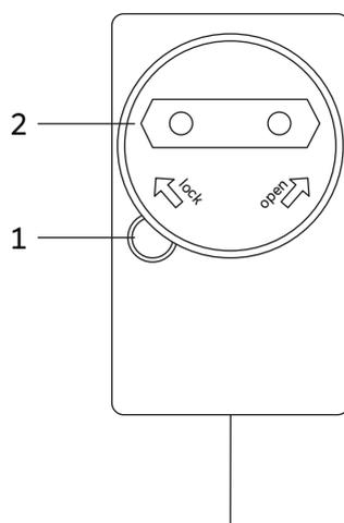
Press the locking button (1) and keep it pressed. Meanwhile, turn the adapter plate (2) counterclockwise to remove it from the power supply.
